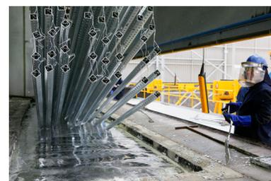
*Post-galvanized EN ISO 1461 is applied after fabrication of steel components to ensure complete coverage of the coating.*
